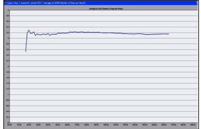
Figure 5.7 Average Hop count per route in scenario 2 with wormhole attack
