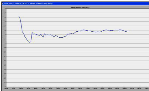
Figure 5.5 Average delays per route in scenario 1 without wormhole attack
