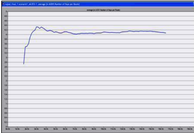
Figure 5.4 Average Hop count per route in scenario 1 without wormhole attack
