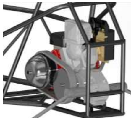
Fig -2: Inclined CVT Assembly
