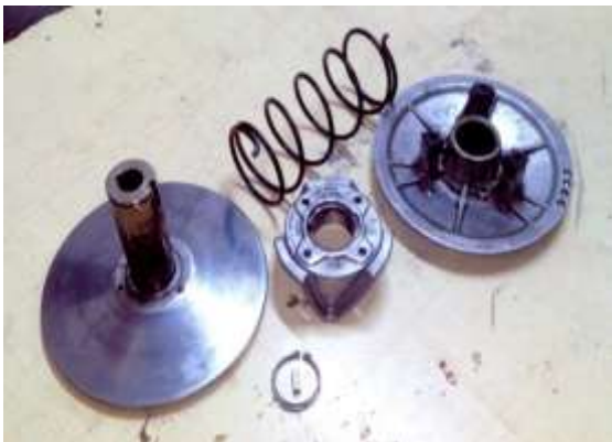
Fig -7: Exploded View of Driven Pulley
