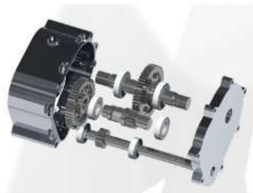
Fig -12: Exploded view of Gearbox 2
