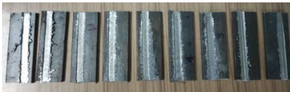
Fig.2: Machined specimens at constant cutting conditions from L9 DOE minimum quantity lubricant (MQL) setup.
