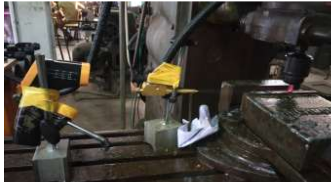
Fig.1: Experimental set-up with a 60 mm of nozzle distance at constant cutting conditions with minimum quantity lubricant (MQL) setup.
