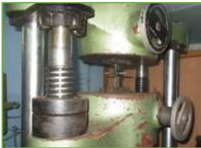
Fig 5. Specimen loaded in UTM machine
