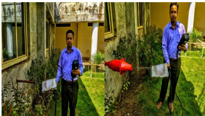
Fig -3: Emissions test before and after using Innovative Catalytic Converter using KIGAZ 310 PRO
