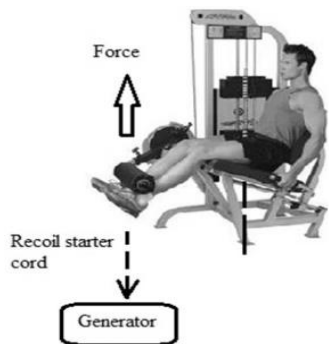
Fig -10: Leg extension machine working as a power generating machine
