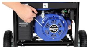
Fig -5: Generator is being started by pulling recoil cord
