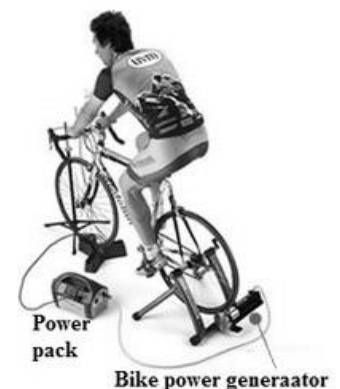
Fig -13: Stationary bicycle is producing electrical energy
