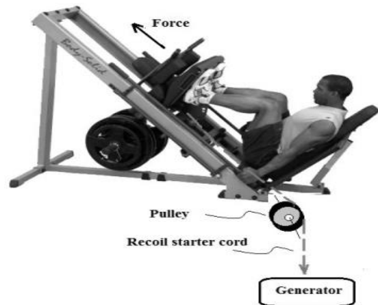
Fig -11: Generator operated by leg press machine
