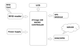
Fig-1: Block Diagram of System
