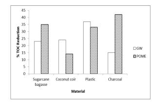
Figure 5: TOC reduction for different media
