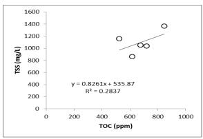
Figure 8: TSS versus TOC for greywater
