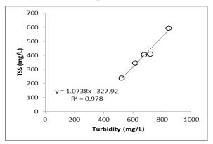
Figure 7: TSS versus Turbidity for greywater
