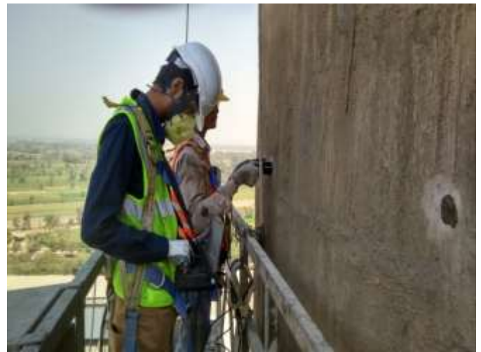
Fig -6: Performing UPV Test at Certain Height
