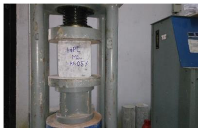
Compressive strength test
