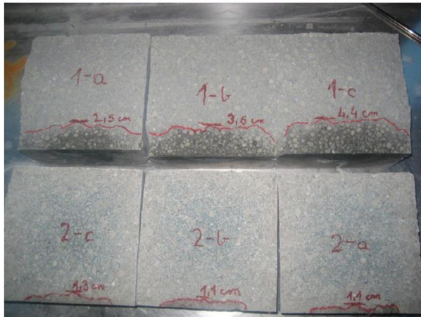
Fig -2: split surface of cubes after water pressure permeability test (Mix A, Mix B )
