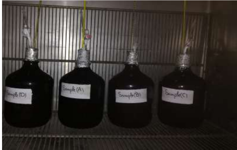
Figure 2 Experimental set up for co-digestion
