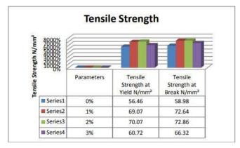
**Chart-1:** Relation between Tensile Strength and wt % of Fly ash
