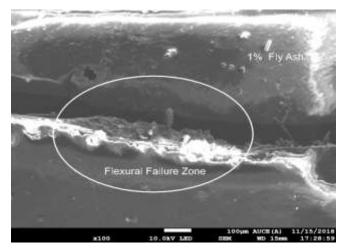
Fig-2: Failure zone of laminate with 1 wt% of Nano fly ash
