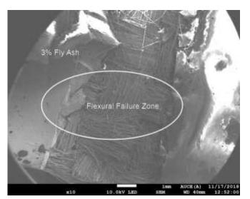
Fig-3: Failure zone of laminate with 2 wt% of Nano fly ash
