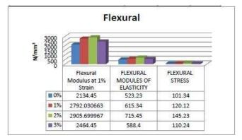
**Chart-2:** Relation between Flexural Modulus and wt. % of fly ash
