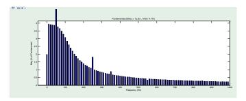
Fig. 5: THD spectrum of Source Current of phase- C with PID controller
