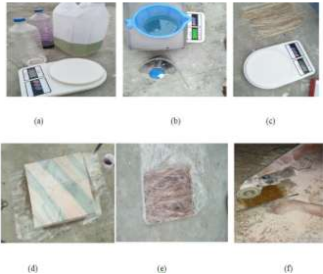
(a) Material (b) weighing of polymer (c) weighing of natural fiber (d) composite sheet under the pressure (e) Prepared composite sheet, (f) Cutting of composite sheet into desired specimen
