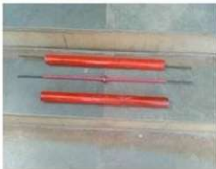
Photo-1: Circular steel core rod wrapped in bond breaking layer and splice placed at the centre of the rod.
