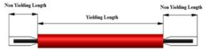
Fig -2: Side view of BRB
