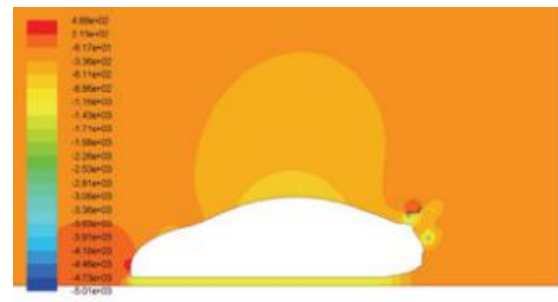
Figure 8: Static pressure contours over the redesigned car geometry (case two)
