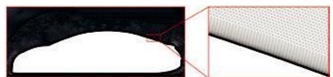
Figure 3: Finite volume mesh of the first case of car geometry (initial car geometry).
