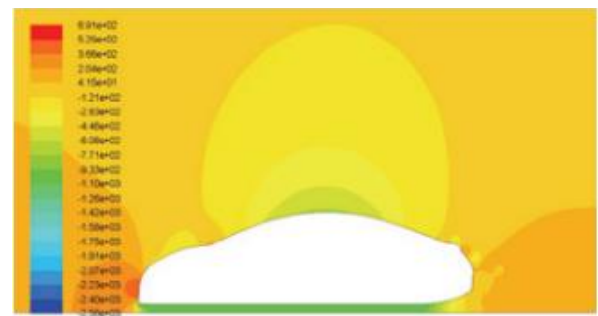
Figure 7: Static pressure contours over the initial car geometry (case one)
