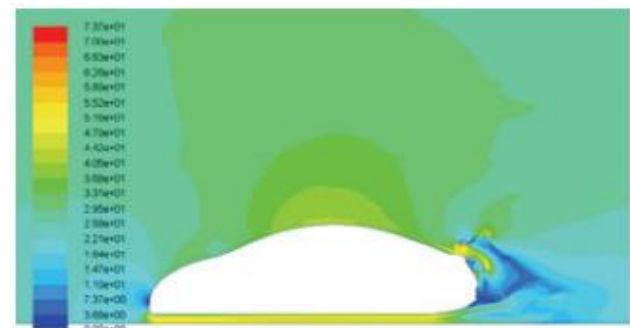
Figure 6: Velocity contours over the redesigned car geometry (second case)
