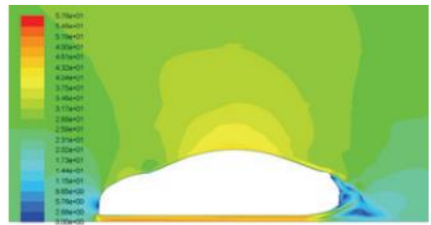
Figure 5: Velocity contours over the initial car geometry (first case)
