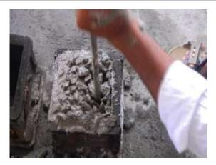
Fig -2: Casting of Cube Moulds
