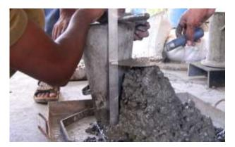
Fig -4: Measurement of Slump
