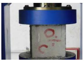
Fig -6: Failure of Concrete Specimen
