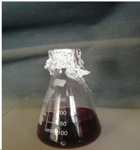
Fig -1: aged solution of silver nanoparticles the reaction mixture continuously for 5 minutes, it was settled to age for 1.5 hours. [15].
