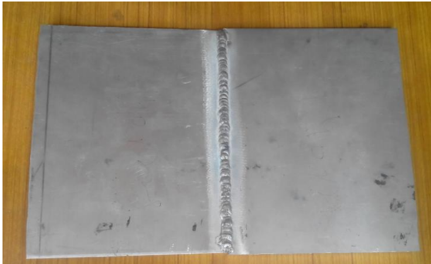
Figure 4 : Welding Plate after TIG Welding at the value of current as 140 ampere
