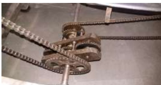
Fig.8: Components of energy flywheel
