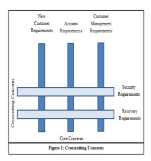
These additional requirements are crosscutting concerns, because these concerns have an impact on other core concerns. In Figure 1, all the core concerns are shown as vertical columns and the crosscutting concerns are shown as horizontal bars that cross the vertical columns. The crosscutting concerns are the main point of interest of an AOP.
