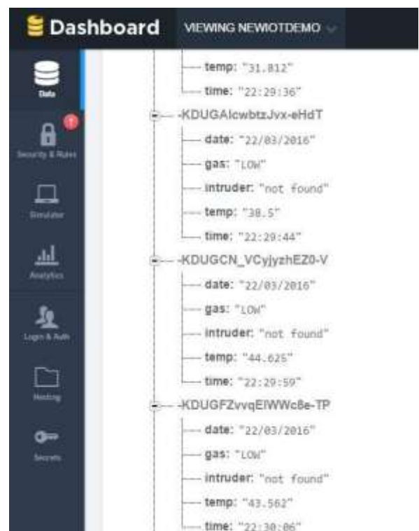
Fig.2.2 Temperature, gas and IR sensor outputs in IOT.
