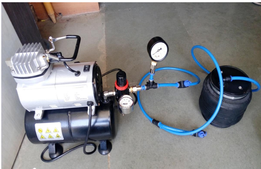
Figure 15: Testing of Air Spring (Single Convolution Bellow) with Compressor and Sensors
