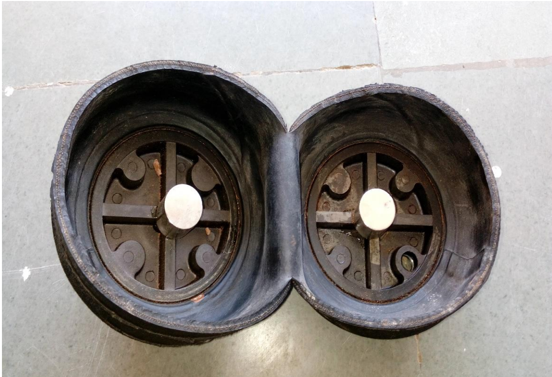
Figure 14: Neodymium Magnet N52 fixed on each end of the bellow (like poles of magnets are placed towards each other to produce repulsive effect)
