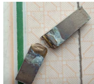
Test Image of Material after Testing in Charpy Pendulum Impact Test
