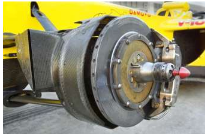
Fig -7: Formula1 brake disk made of carbon -carbon composites
