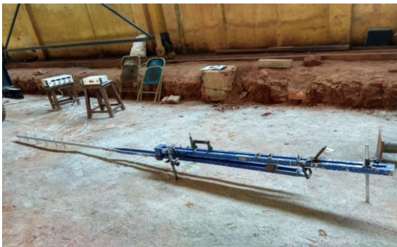
Fig-12: Modified Benkelman beam with fixed LVDT's
