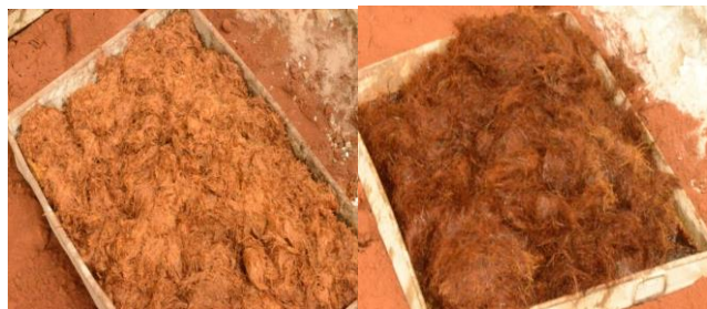
Fig-2: NaOH treated Jute and Coir Fiber
