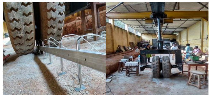
Fig-13: Position of LVDT's and position of Dual wheel assembly with jack
