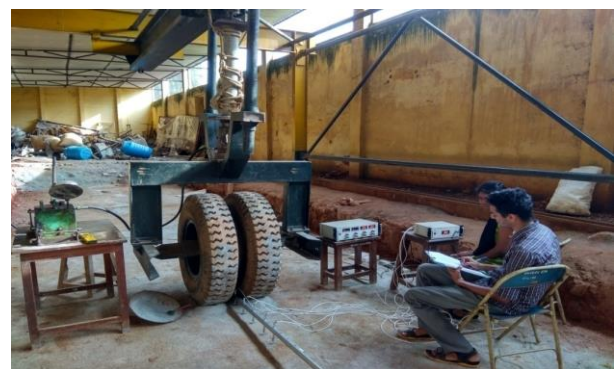
Fig-14: Dual wheel load test setup
