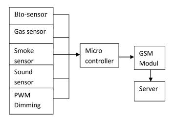
The data from the Bio sensor, Gas sensor, Smoke sensor, Sound sensor, And PWM dimming is sent to the micro controller which controls the recording or it intimidates the information and the data is sent to GSM module which maneuvers the street lamping system the main work of the system is to get the information or record the information and send the same to the main server.
