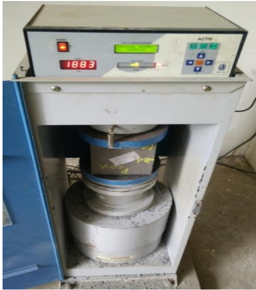
Fig -6: Compressive testing
