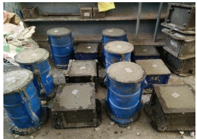
Fig -4: Casting of geopolymer concrete
