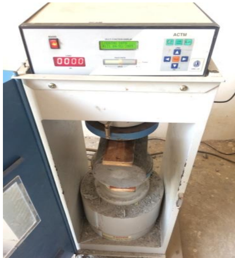
Fig -7: Split tensile testing
