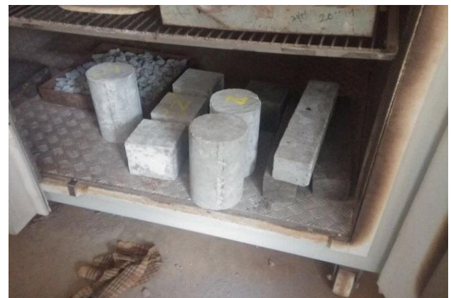
Fig -5: Thermal curing of geopolymer concrete
