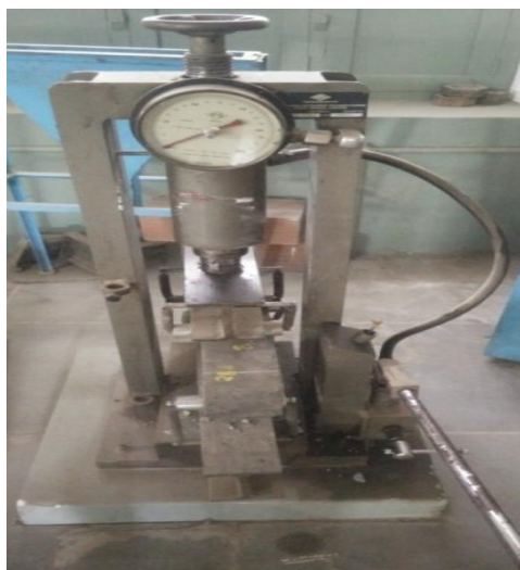
Fig -8: Flexural testing
