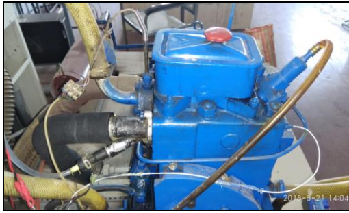
Fig.1 : Intake Port Fuel Injection
