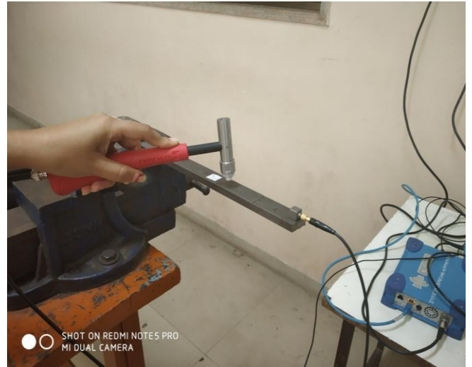
Figure 10 : Experimental Setup Using FFT Analyzer
