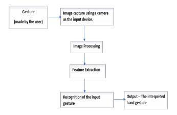
The gesture made by the user is received through the camera. The image is then processed for extraction of its features. The collected data is then used for further calculations. It is compared with the existing data set and recognized. The interpreted gesture is then given as the output and then used for the required purpose.
