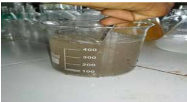
Fig 2: Sample for salt ponding test
