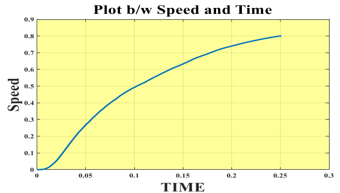
Fig-3.2.1 (a): Graph b/w speed & duration with P controller when K_{pL} = 0.009 ,
