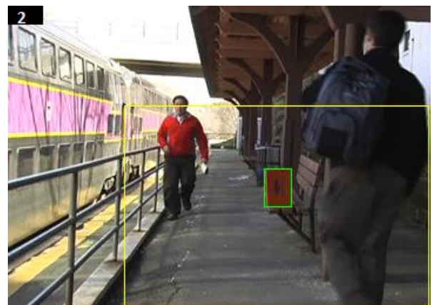
Figure 3(b). Output image – abandoned object detected
