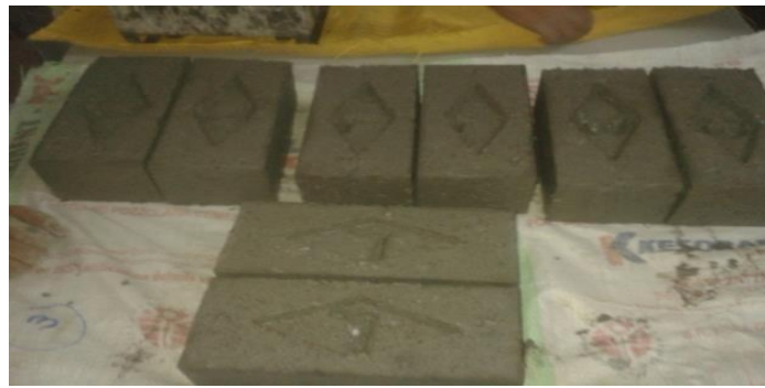
Figure-2: Casting the papercrete brick [9]
