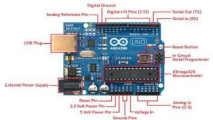
Fig-3: The outer look of the Arduino UNO board
