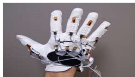
Fig 4(b). Exoskeleton hand robotic training device.
