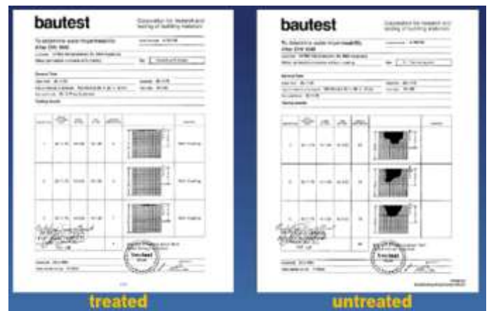
Fig. 19: DIN-1048 permeability test
