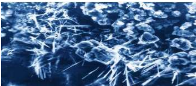
Fig. 14 By-products of cement hydration precipitate in capillary tracts + Crystalline reactive chemicals = Crystalline initiation
