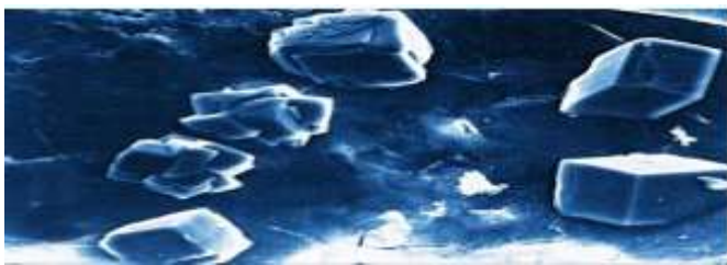
Fig. 13: Scanning electron microscope (SEM) view of a concrete pore filled with multiplicative crystalline formation, initial stages
