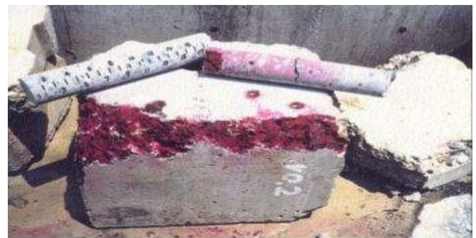
Fig. 16: Crystalline waterproofing on concrete surface
