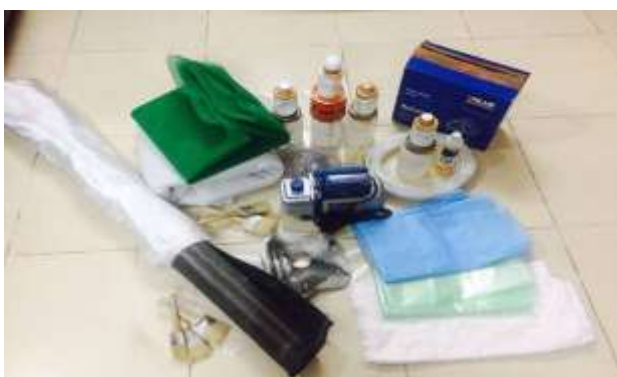
Fig 7. Fabrication kit vacuum bagging.
