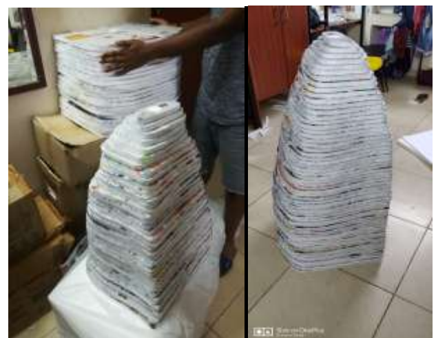
Fig 5. Nose cone mold without finish.
