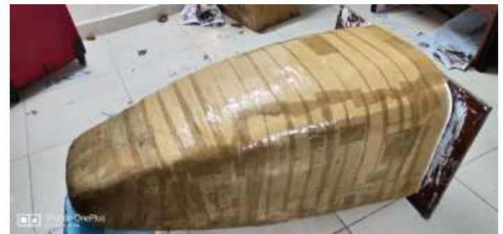
Fig 8. Mold with taping.
