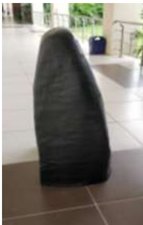
Fig 10. Different views of final product-Nosecone. Final Weight was found to be 1.7 KG
