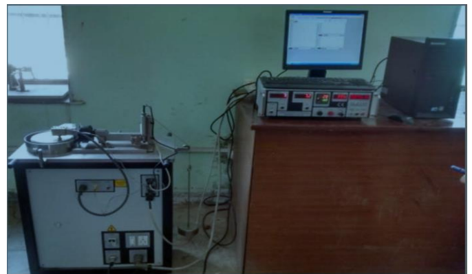
Fig 8 : Pin on Disc set-up
