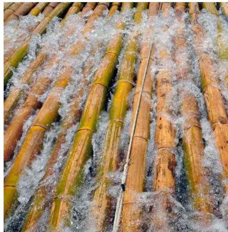
Fig -1 : CCB Treatment of Bamboo
