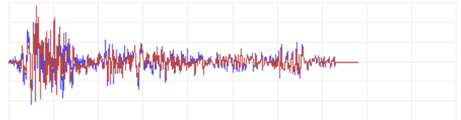
Fig -5: Time History function matched to Codal spectral function in Time domain using ETABS 2015
