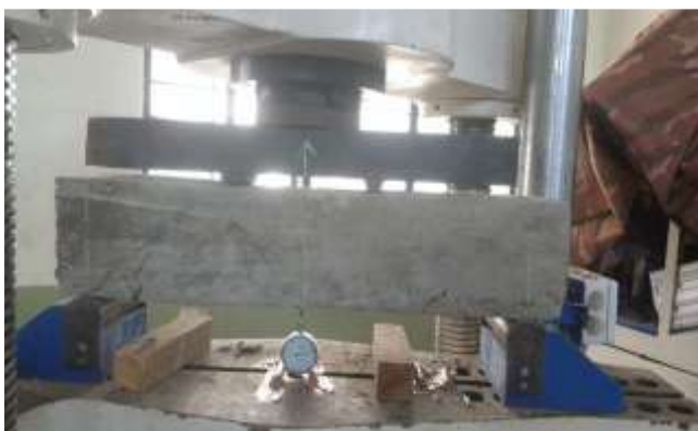
Applying a load on deep beam
