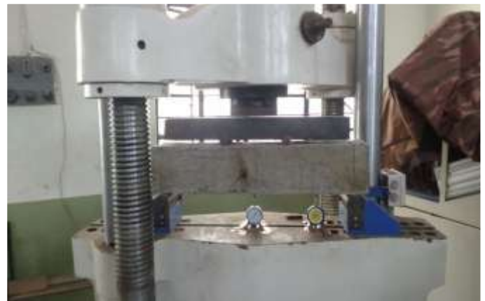
Flexure failure shows in beam
