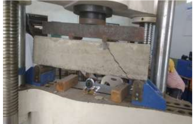
Shear failure and cracks on beam
