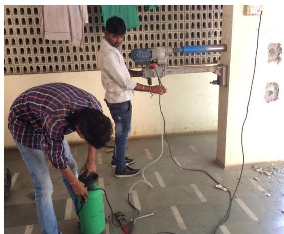
**Concrete Core Test**
