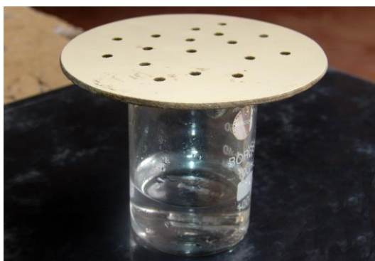
Figure 1 Photograph showing the simplest apparatus to grow crystals using slow evaporation technique.
