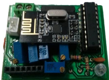
Fig. 6. The Sensor board: Micro-controller, conditioning, Radio, with the dimensions of 55x45mm.
