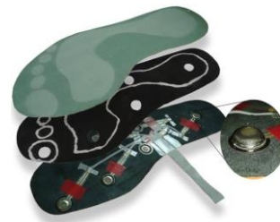
Fig. 3. Layers of the insole
