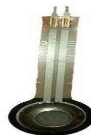
Fig. 4. Modified force sensing resistor
