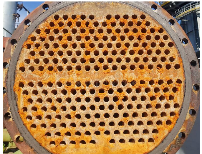
Fig.1: Fouling in Shell and Tube Heat Exchanger
