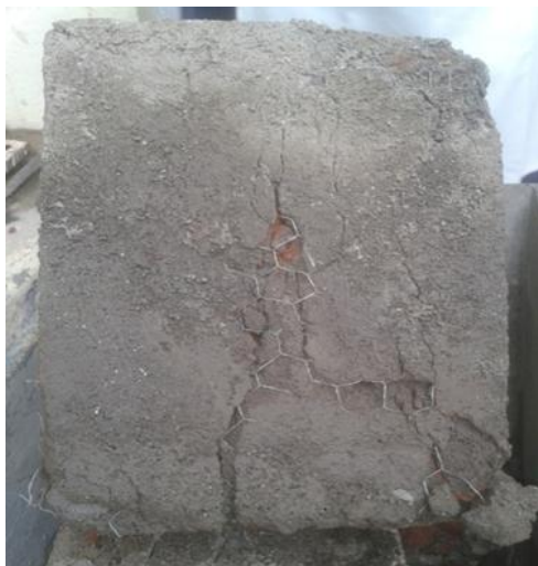
Fig 4) CRACKING OF FERROCEMENT COLUMN (1:2)
