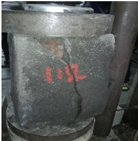
Fig 3) CRACKING OF PLASTERED BRICK COLUMN (1:2)
