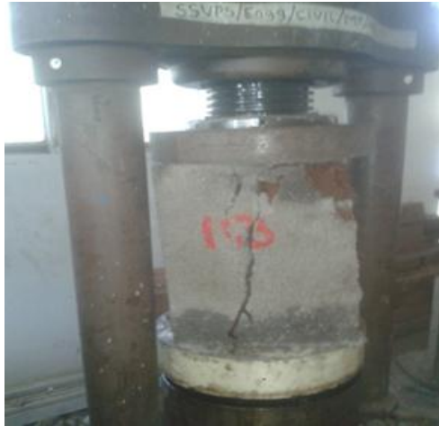
Fig 2) CRACKING OF PLASTERED BRICK COLUMN(1:3)
