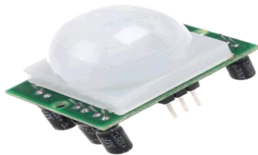
Fig 4.1.1 Passive Infrared Sensor
